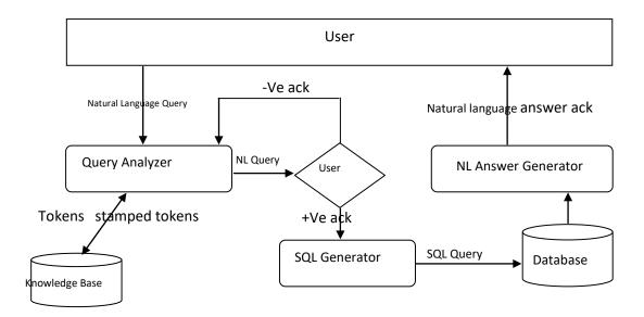
Fig: Architecture for QA System
