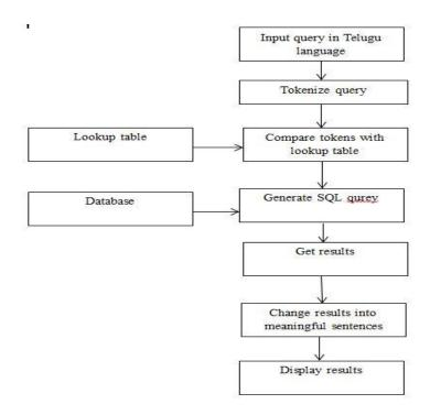
Fig: Block diagram for QA System
